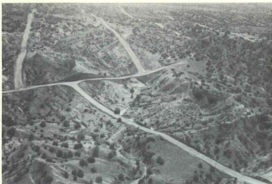
Santa California City, an area near State Roads 84 and 96 in Rio Arriba County. The roads were constructed in 1970 with NO regard for drainage.
